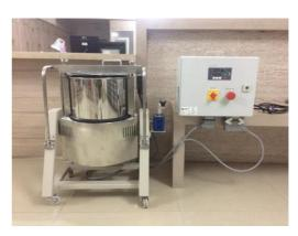
These machines are the perfect companions to work with. The Nemisto melangeur is included with a control panel which consists of an emergency stop, speed indicator, timer and start / stop buttons.
