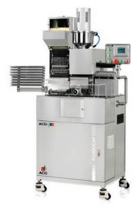
The Fluidocap 1000 is a semi automatic, laboratory machine that can fill liquid into hard capsules and band-seal them using a gelatin band.
