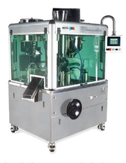
The Fluidocap F40 and Fluidocap F70 are fully-automatic capsule-filling machines that can fill a large variety of liquid and semi-solid formulations into two-piece hard capsules.
