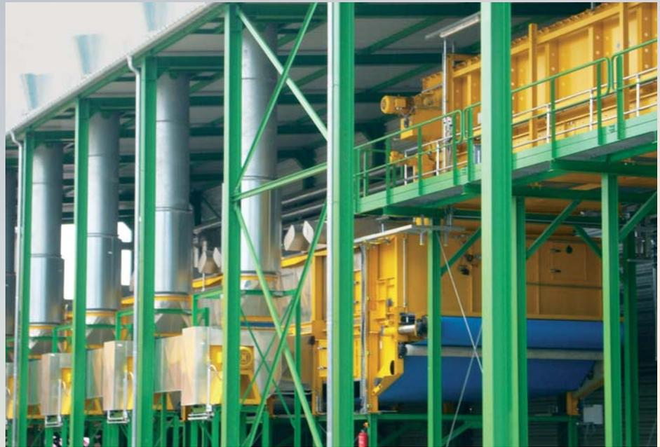
The fabric belt drier in a wood pelleting plant
