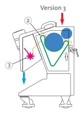
This version will roll out the hot melt into a thin film. The product is then pressed with a belt ② (green) against the cooling drum and can be efficiently cooled and solidified with a long active cooling path. The solidified product is then guided to the flaker ③ (magenta) where it will be broken down into homogenous flakes.
