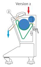
This version will roll out the hot melt into a thin film. The product is then pressed with a belt ② (green) against the cooling drum and can be efficiently cooled and solidified with a long active cooling path. The solidified product is then guided to the product outlet.
