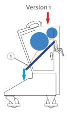
This version will roll out the hot melt into a thin film which will be cooled on a short path between the two drums. A cooled product chute ① (dark blue) is then guiding the solidified product to the product outlet.
