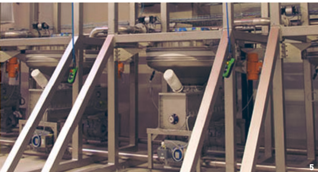
1 System to reuse Big bag 2 Extraction with vibrating cone 3 Chain hoist to load bags 4 Vibrosifter 5 Multiline feeding 6 Antidust filter
