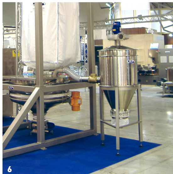
1 System to reuse Big bag 2 Extraction with vibrating cone 3 Chain hoist to load bags 4 Vibrosifter 5 Multiline feeding 6 Antidust filter
