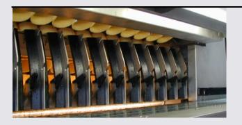
Bottle output with one-finger-system. The bottles are discharged from the cells without any fall! Pushing over with parallel continuos delivery table guarantees high stability.
