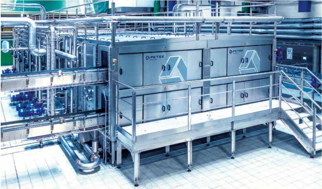
Tunnel technology is a complex system which can combine several functions (pasteurization, re-cooling, warming) and can be quite a big user of energy for heating and cooling. Therefore, to be able to follow all these high demands we are in-building central hot water unit in combination with water saving system.
