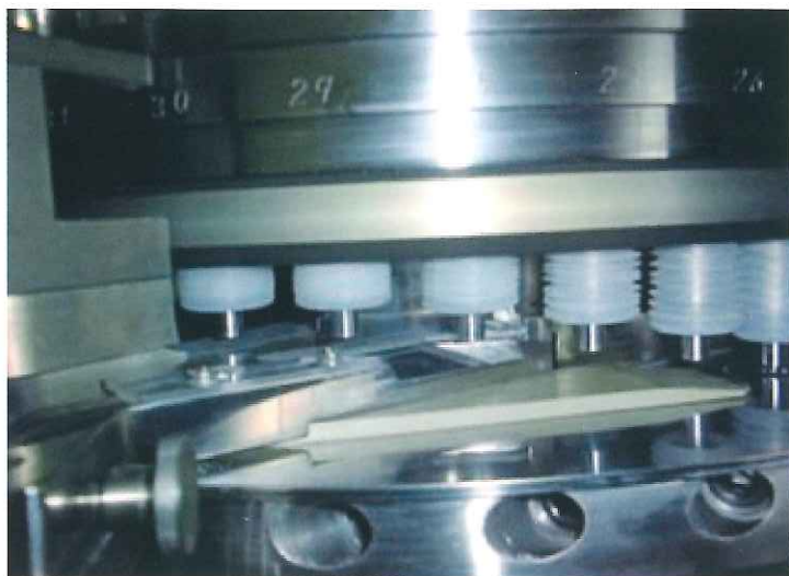
Upper Punch Dust Seals & Bellows
