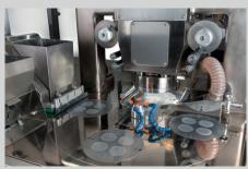
Automatic hopper for depositing cosmetic powder into the pans. The powerful brushless motor combined with the new dust shaking system speeds up the phase of spreading the product in the cavities of the mold. The quick release of the hopper facilitates the cleaning and sanitizing operation for each product change.
