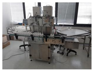
All parts in contact with products are in stainless steel AISI 316L, food grade plastic material and crystal glass.
