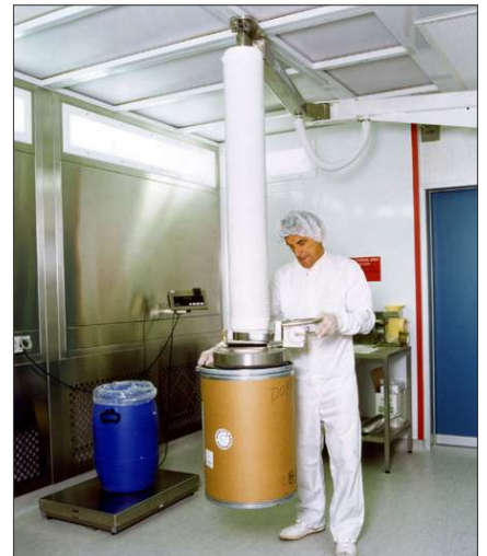
PalPharmaVac™ handling fibre drums, plastic kegs and sacks supported from a 3m (10') stainless steel ceiling mounted articulated crane. PalPharma Handling Solutions unique low headroom hygienic lifter ensures the operator can achieve the required lift heights within restrictive environments as shown above in a downflow booth.
