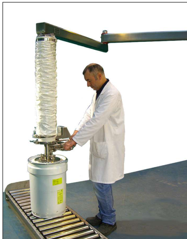
Ceiling mounted articulated arm with 360° continuous rotation. Used to lift various fibre drums from a pallet to a conveyor weighing 60kg. The drums enter a containment booth where the product is dispensed. Suction foot has a flat seal for smooth lids shown loading a PALPharma cGMP roller conveyor which fed into a PalPharmaTip
