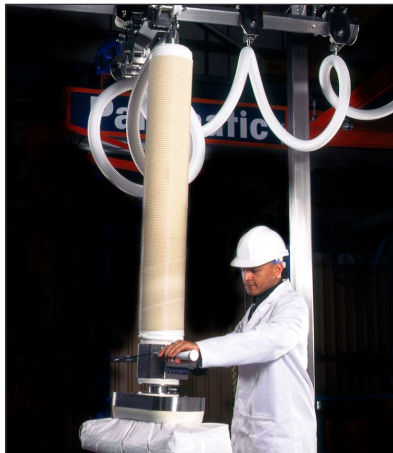
PalPharmaVac mounted on a cGMP stainless steel crane system with all moving components externally mounted for easy clean down and maintenance. Rollers bearings are made from non particle shedding co-acetal polymer. The rails are suspended build up that there are no flat surfaces to allow dust build up. The crane system is available with a variety of finishes and sizes to suit all budgets.
