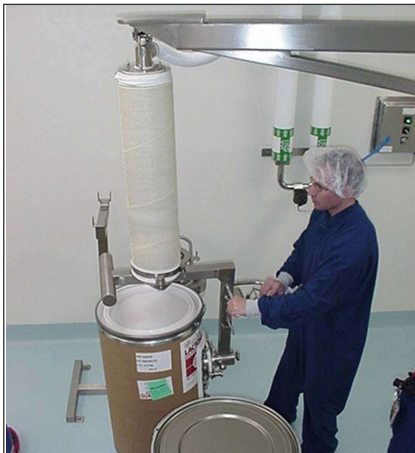
PalPharma Vac™ installation in USA to side lift drums with a simple pin lock out rotation, within a weighing area.
