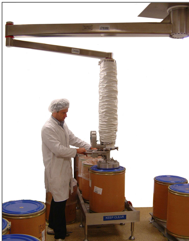
Ceiling mounted articulated arm with 360° continuous rotation. Used to lift various fibre drums from a pallet to a conveyor weighing 60kg. The drums enter a containment booth where the product is dispensed. Suction foot has vertical type seal for lifting lids with indents and ridges
