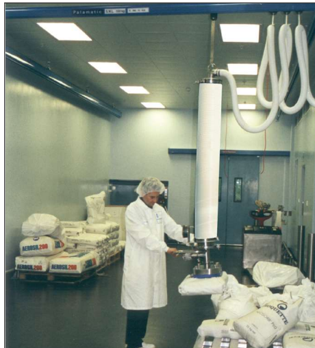
PalPharmaVac™ handling sacks, drums and boxes up to 50kg in a batch assembly area. The PALPharmaVac™ is mounted from a ceiling supported crane gantry measuring 20x4m. The products are lifted from dirty pallets on one side of the room to clean pallets on the other.
