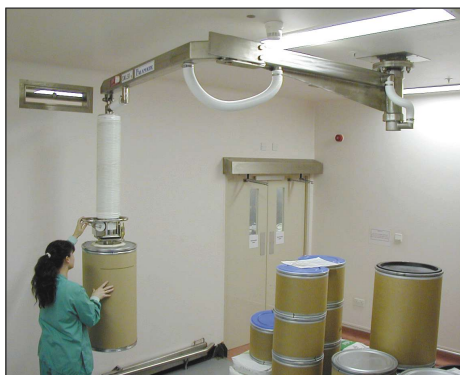
Fibre keg, plastic drum and sack handling PalPharma Vac™ supported from a ceiling mounted 360° rotational articulated arm, manufactured in 304 stainless steel.
