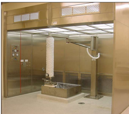
Installation in Puerto Rico. Interchangeable end effector to lift sacks and pour drums within a containment booth
