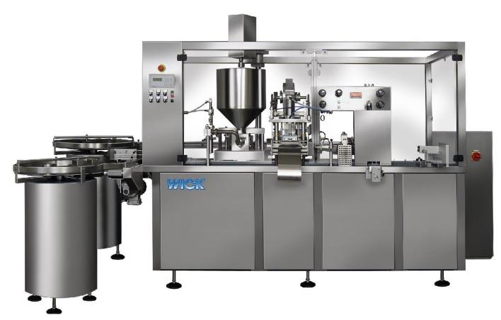
Machine design: indexed inline filler and capper with 1-8 lines
