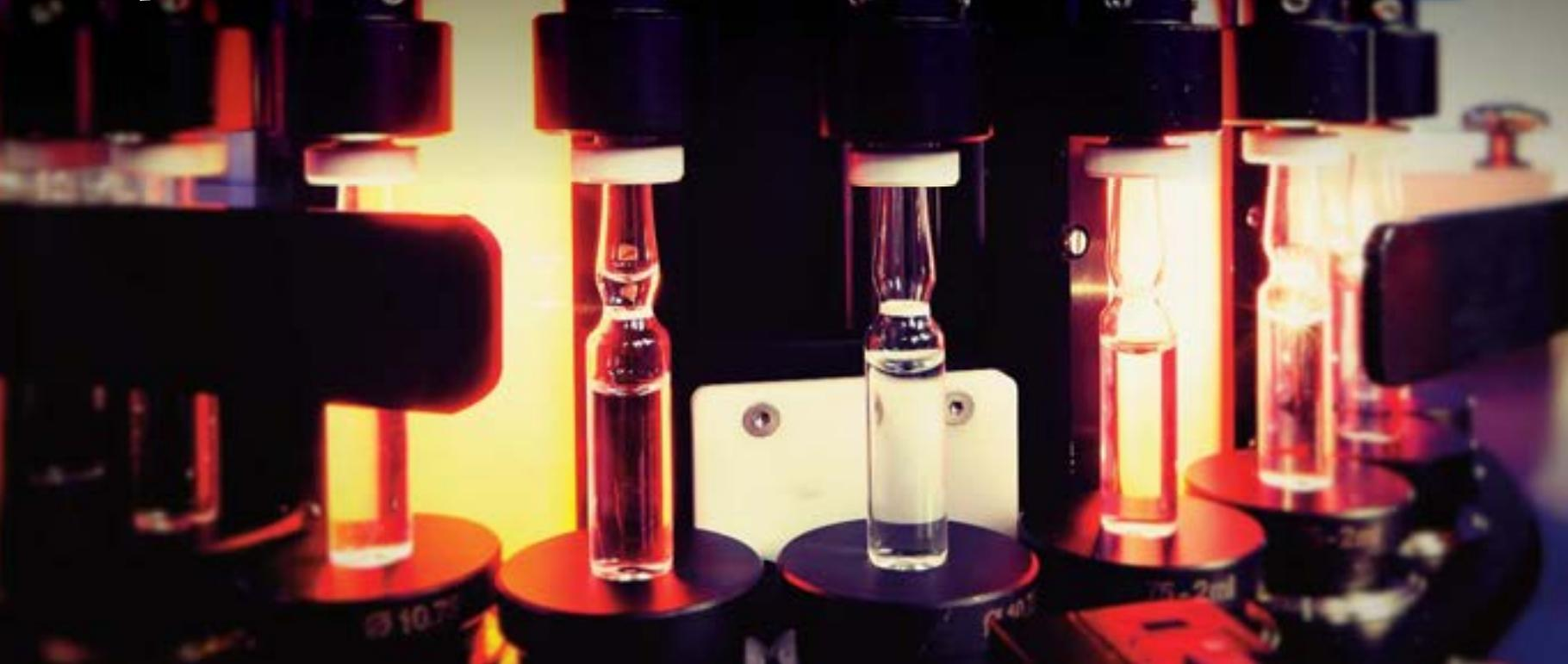
CMP inspection machines by TV cameras and magnifying lenses:
