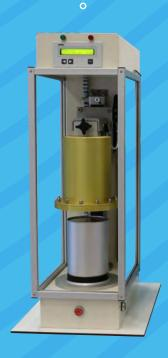
The CLT measures according to the non-destructive detection of leaks in packages by the vacuum decay method (ASTM F2338).
