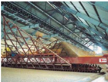
*Bridge reclaimer for limestone (cement plant)*
