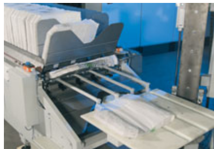
Fully automatic feeding of the empty bag bundles – high productivity is guaranteed
