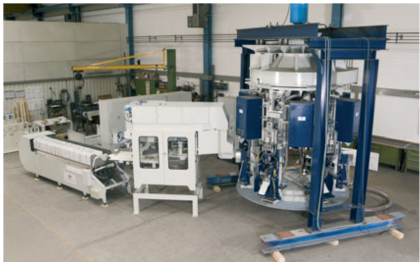
6-spout air-rotary packer with bag applicator and cassette magazine during testing in works.
