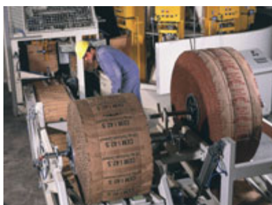
The double reel magazine allows the change of rollers with ongoing filling
