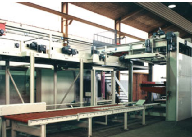
Palletizer with pile-up line for filled pallets, served by forklift
