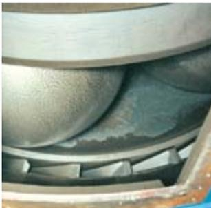
EM Mill grinding elements.
