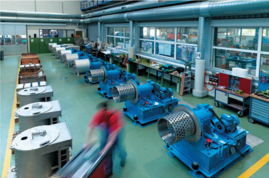
Pusher centrifuges P-50, sodium sulphate/Glauber's salt
