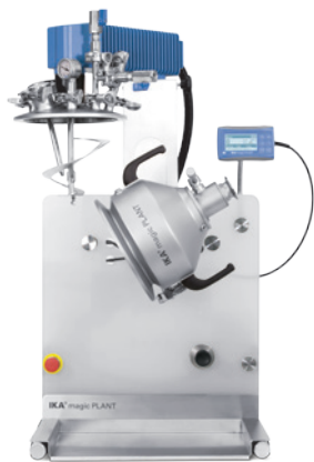
Discharge by complete tilting of the vessel
