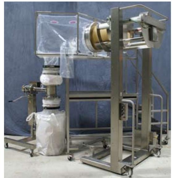
Figure 1b – Variable Height Lifter
