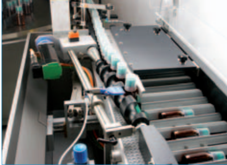
Auger transfer of bottles
