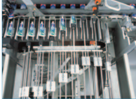
Gentle, continuous product loading stroke. Leaflet pre-insertion into the carton for up to 50 mm loading depth.
