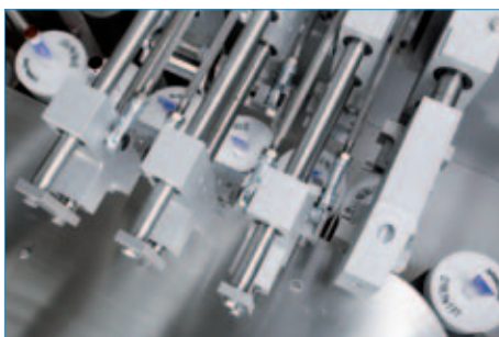
Modular folding and press station for metal tubes with double, triple or saddle fold
