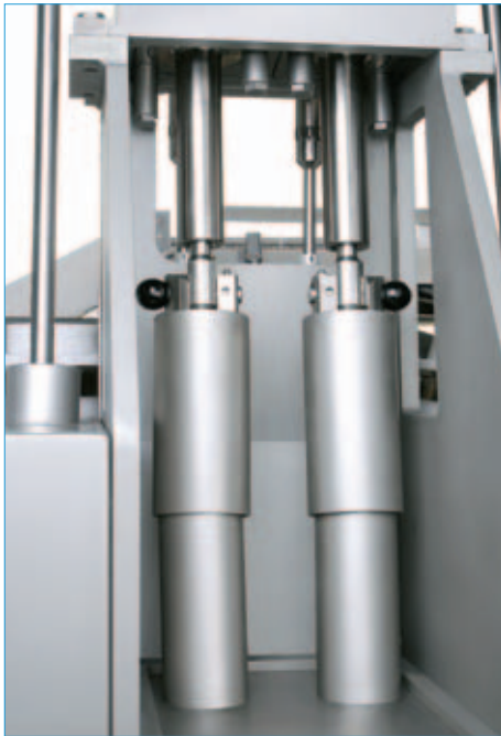
Fast exchange of rotary valves in the filling station, TFS 80-2
