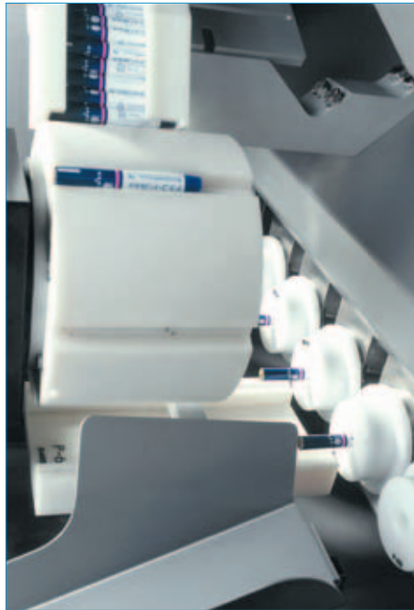
Tube feeding by servo driven loading drum, TFS 80-2
