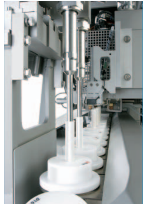
Servo driven transport system for precise positioning, TFS 80-2
