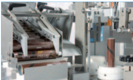
Tube feeding conveyor – chute – rotary machine table
