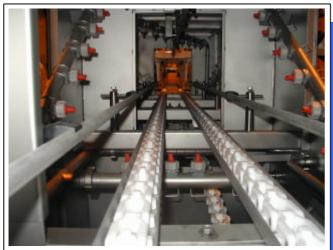
The cases are cleaned reliably from all sides. The clampable cone nozzles are adjustable within a wide range and can thus be adapted to the special characteristics of the cases. Narrow chain conveyors ensure excellent cleaning also from below.
