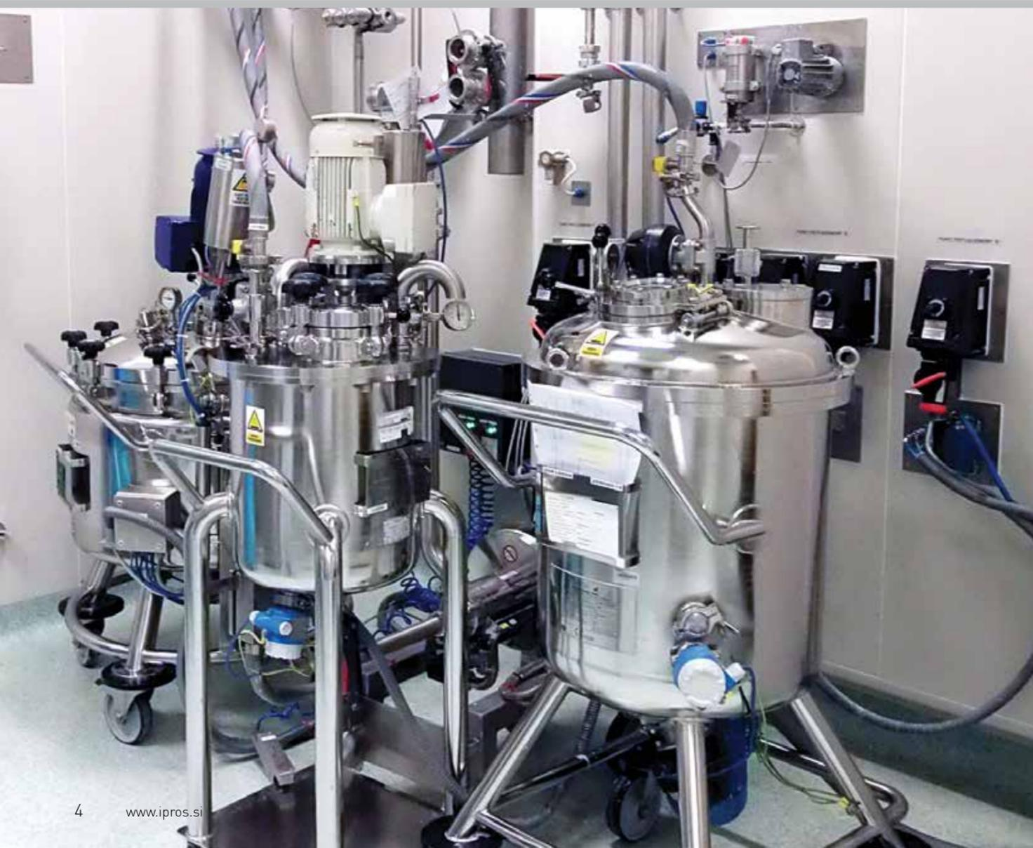
Vessels can be equipped with cooling and heating elements, they can be non-insulated or insulated with insulating material and an insulating jacket (made of stainless steel AISI 304 or other materials) with integrated agitator and other equipment based on order specifications.
