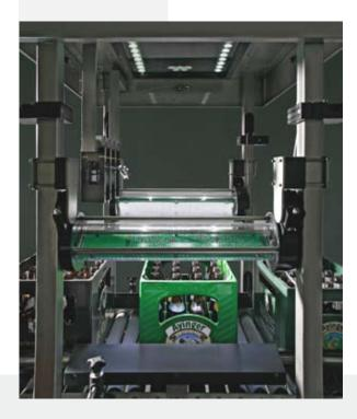
miho Maxx is a Crate Inspection Machine that monitors and sorts empty crates in accordance with different criteria achieving a level of performance that exceeds any level reached up until now.
