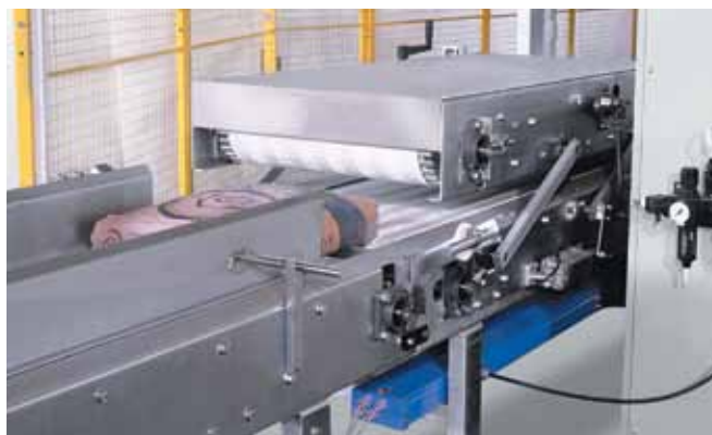
Bag pressing device acting as bag flattener with damping device
