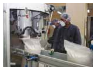
The bag is transferred in the upright position into the bag closing device
