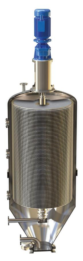
The FUNDA® Centrifugal Disc Filter is a totally enclosed pressure filter with horizontally arranged, self- supporting filter screens for pre-coat or residue filtration of large quantities of diluted suspensions in an automated, closed system. Heel volume filtration to minimize product losses. Cake washing in cascade operation.
