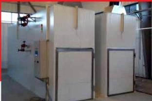
Drying machine consists from drying chamber and air duct system on the top of the "product flow".
