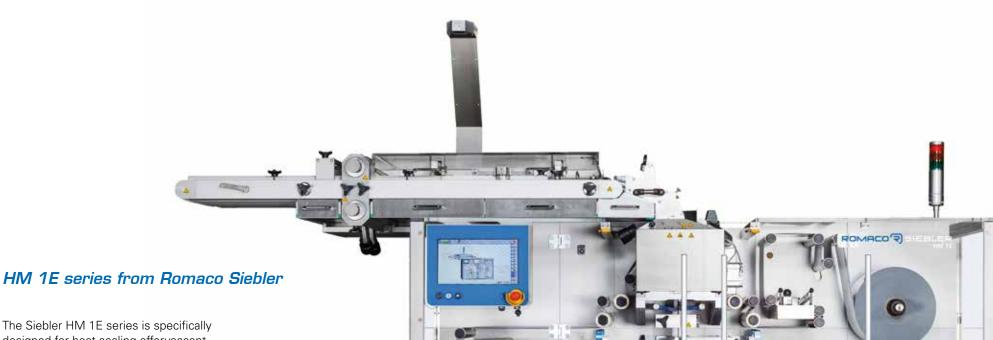
The Siebler HM 1E series is specifically designed for heat sealing effervescent tablets, a highly sensitive product that requires the best possible protection against humidity. The sealing parameters comprising pressure, temperature and speed are preset and stored as format parameters for the relevant products. For contract manufacturing companies or customers with different pack sizes the new sealing system with pluggable tubular format tools is a perfect solution.
