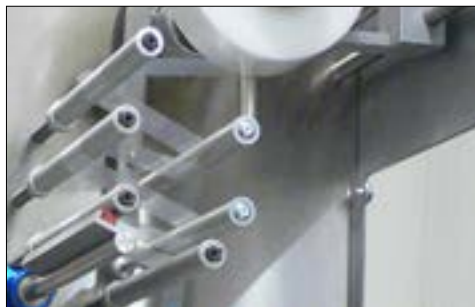
Strain release during foil unwinding
