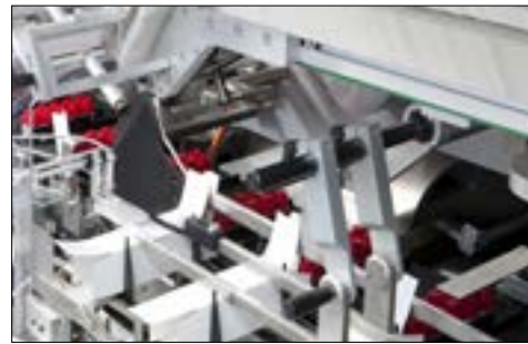
Product feed into the open cartons
