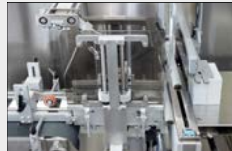
Stacking unit and hot sealing bar
