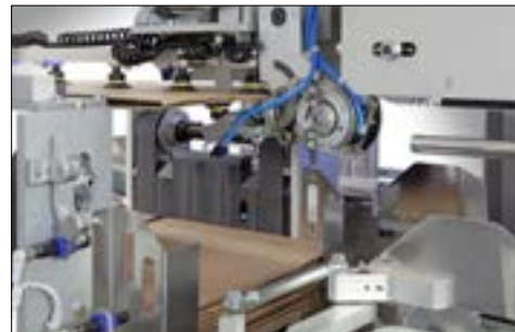
Automatic case erection
