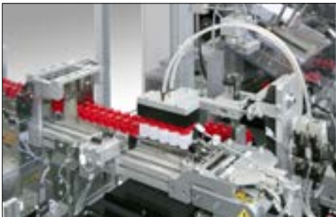
Bottle feeding into bucket chain
