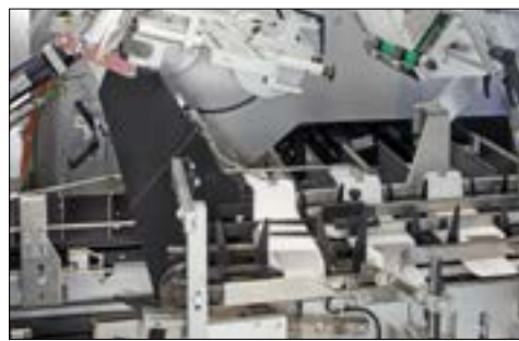
Product feed into the open cartons
