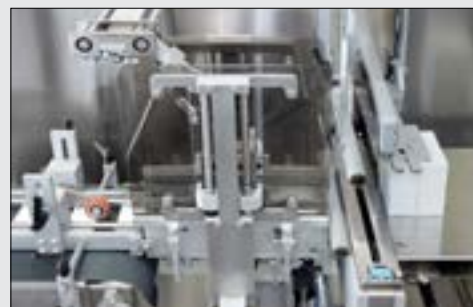
Stacking unit and hot sealing bar
