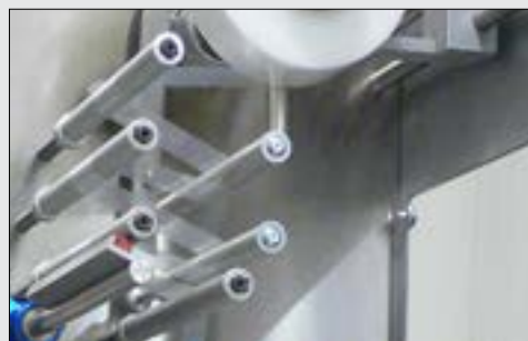
Strain release during foil unwinding
