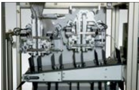
Stacking into the bucket chain
