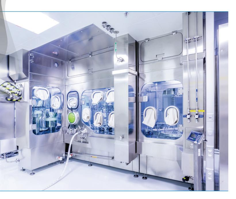
STERILINE closed Restricted Access Barrier Systems (cRABS) are designed for the production of sterile products, either toxic or non-toxic. These systems provide protection for operator from product and for
