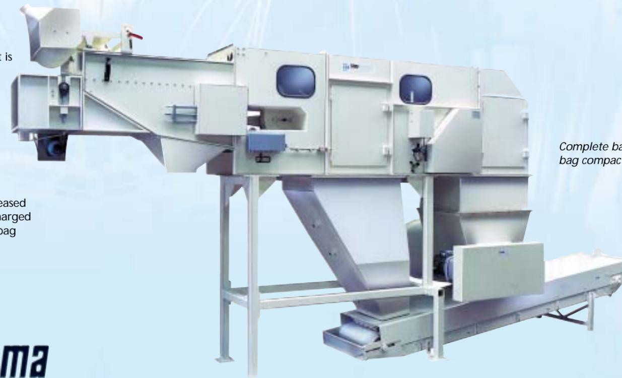
Complete bag slitting machine with cleaning unit, bag compactor and enclosed belt conveyor
