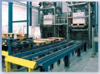
Big-Bag filling system for handling resin flakes
