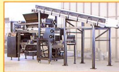
NASTRO CONVOGLIAMENTO IMPASTO A ESTRUSIONE CONVEYOR BELT OF THE DOUGH TO THE EXTRUDER
