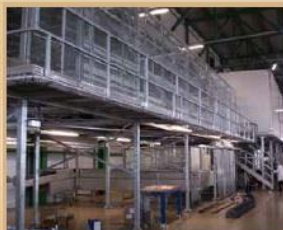
CELLA A BILANCELLE CELL WITH PIVOTED-PLATES
