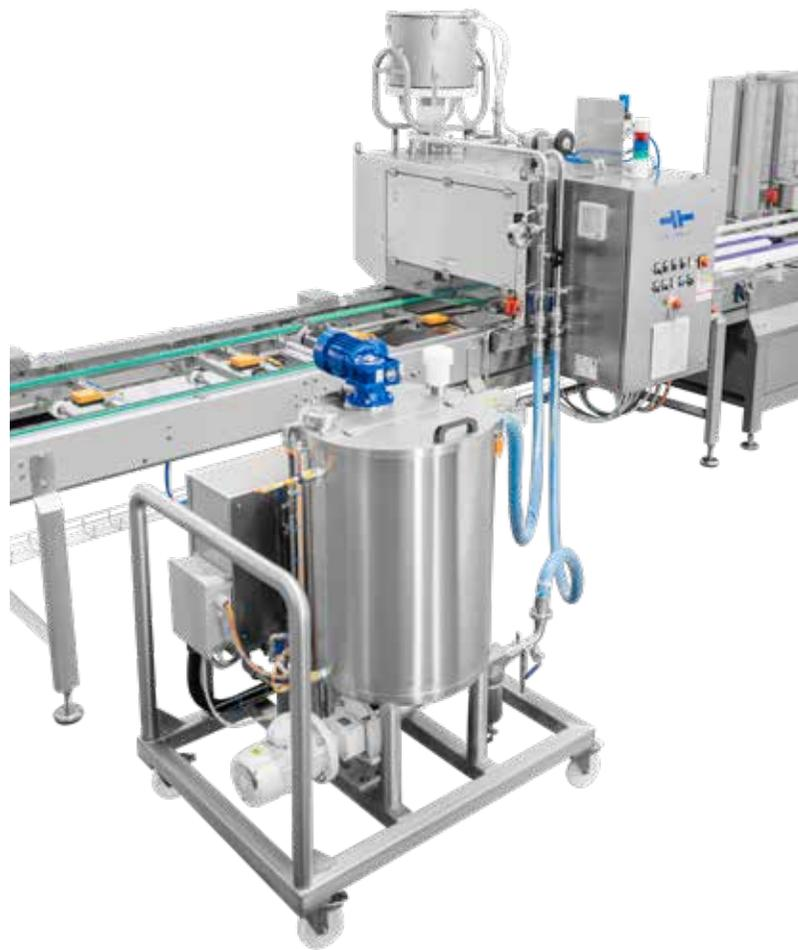
Machine designed to accurately grease the product cavities in the baking trays, parametrizable with PLC control. The specific engineering of our machine allows an effective extraction of the cake during the depanning operation, reducing downtime and waste. Greasing agent pressurized loop, with recirculation to the temperature controlled tank. Centrifugal fumes extraction system.
