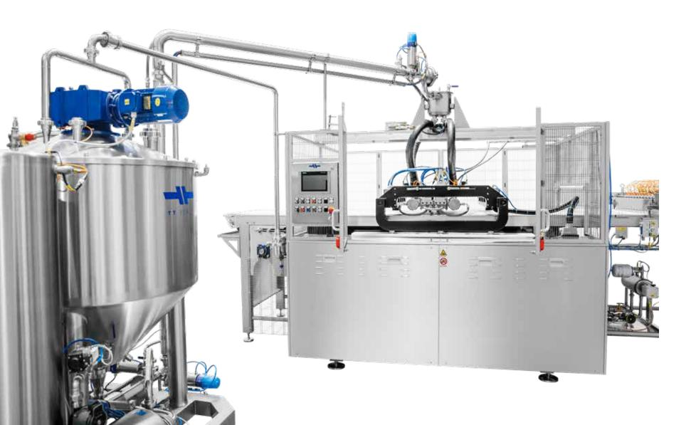
TT Italy's Topping Machine is designed to accurately dose toppings onto your product, while it is moving on the conveyor belt. Our tailor-made solutions cater to all productivity volumes and formats.
