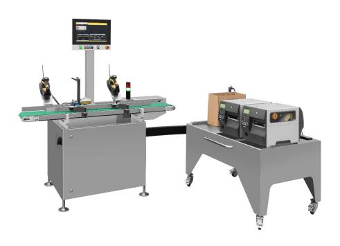
With Trackpca, it is possible to print and control variable data and codes on cartons of different formats, even non-serialized ones and to print and control labels for cases and pallets.
