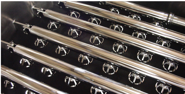
CIP performance of the STERIBAC® system: Filter cover, view of fixed filter parts before and after CIP
