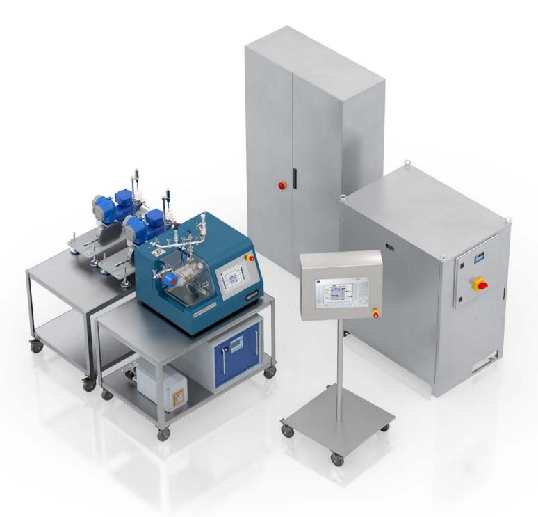
The system allows working in both passage and circulation processes. Processing starts with 1 litre of suspension and can be scaled-up to the larger models of the DYNO<sup>®</sup>-MILL series.
