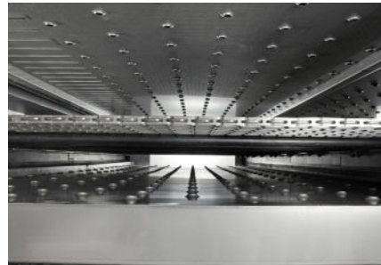
Multibake® tunnel ovens • Impingement technology • Indirect heating & baking
