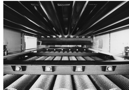
MB-R tunnel oven • Cyclotherm & radiant tubes • Indirect heating & baking
