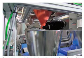
The products are dosed into the target container with an accuracy of up to  $\pm$  2 g (depending on the raw material and flow behavior) via the AZO®eDos dosing system. Advantages: simple geometry, easy to clean, hygienic, easy to dismantle
