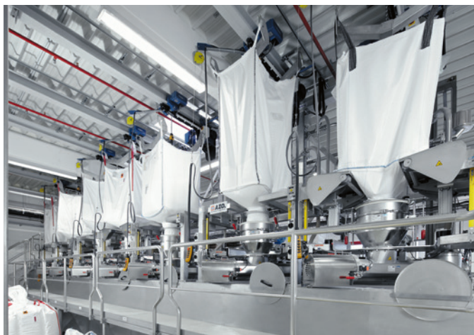
Big bag discharge stations with dosing screws for medium components
