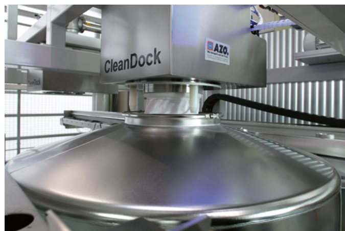
AZO CleanDock® for dust-free docking and undocking of mobile containers
