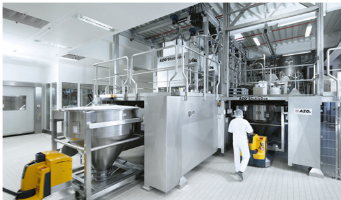
Locking MIXTAINER® containers in and out on the AZO ShuttleDos®
