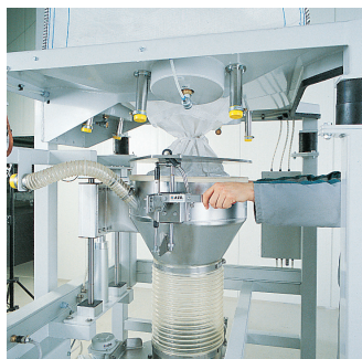
Discharge system raised, with opened clamping disc.
