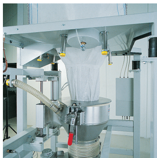
Lowering the connecting system tensions the big bag discharge sleeve. The big bag is now ready for discharge.
