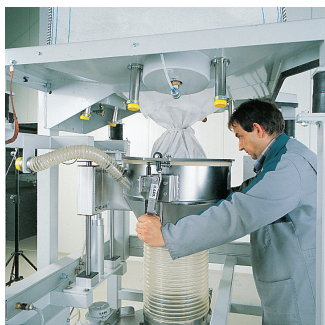
Big bag discharge sleeve connected to discharge tube, and fastened with the clamping disc. Draw string on big bag outlet released.
