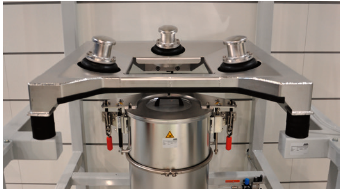
Support hopper with vibrating discharge aid and massager device
